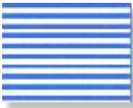
1/8" (3mm) Lines on 1/4" (6mm) Centers - 50% Coverage
